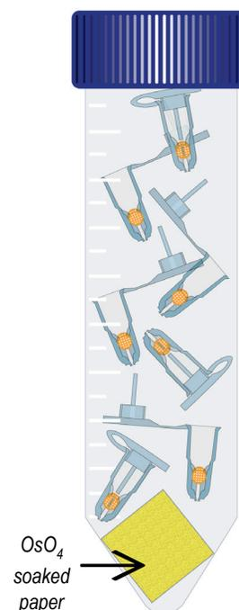
**Figure 4: Decontaminate and transfer to vessel.** Placing virus-loaded grid-containing capsules into a vessel filled with osmium tetroxide vapor can be used to decontaminate viruses. Capping the vessel allows safe transport of the grid-containing capsules into the EM lab.
