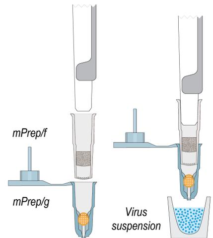
**Figure 1: Set up mPrep/g capsules with grids and apply viruses.** A single mPrep/g capsule containing two grids is attached to a single-channel pipettor via an mPrep/f filter coupler. In practice, identification labels are attached to capsules, and multichannel pipettors can be used to process several grids.
