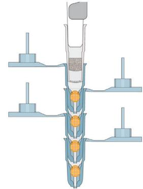
**Figure 10: Stacking capsules to simultaneously process multiple grids.** Inserting 1 or 2 grids per capsule and stacking up to 4 capsules per channel of the pipettor enables processing of many grids.
