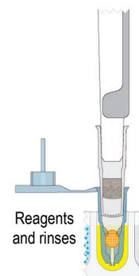
**Figure 2: Transfer viruses and reagents into mPrep/g capsules by pipetting from reagent vessel.** Rest the ends of the capsule(s) in the bottom of microplate wells or reagent reservoirs. Aspirate virus suspensions and reagents into mPrep/g capsules. Use a lab stand (not shown) to support pipettor vertically.
