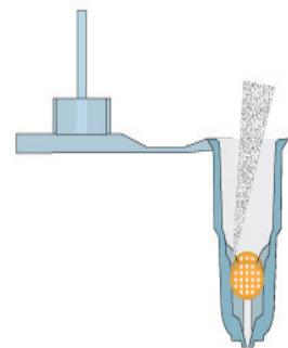
**Figure 6: Blotting grids.** Grids are blotted to remove negative stain and to accelerate drying. Insert a filter paper wedge or other absorbent material into the mPrep/g capsules and touch where the grids are held in the capsule slots.
