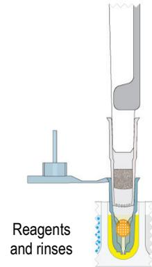
**Figure 5: Deliver stains and labels to the grids in the EM lab.** Rest the capsule end in the microwells or reagent reservoirs to the rinses, uranyl acetate, and any other stains or labels into the mPrep/g capsules.
